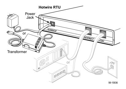
The RTU hardware installation is now complete. When the power cord is installed, the RTU goes through a power-on self-test.
